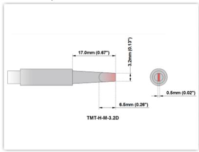
TMT-H-M-3.2D Chisel 3.2mm (0.126")
