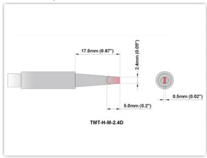
TMT-H-M-2.4D Chisel 2.4mm (0.095")
