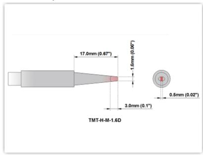
TMT-H-M-1.6D Chisel 1.6mm (0.063")
